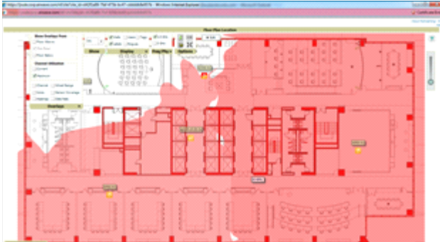
Figure 16 Channel Utilization in VisualRF (Interference)
